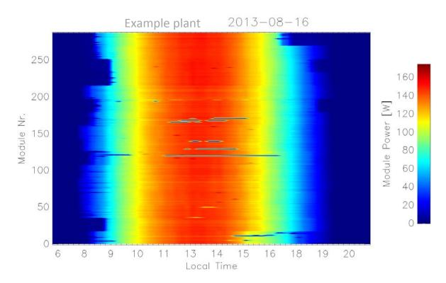
The system automatically recognizes a cloudless day and provides the corresponding analysis. A basically well-functioning plant can be seen in the example given here. However, a few "inclusions" can be discerned: the bar in the middle, for example, or the formation at the bottom right. This formation nicely shows a wandering shadow - a lamppost, maybe. The central bar on the other hand indicates that the corresponding modules malfunctioned during the midday period.
