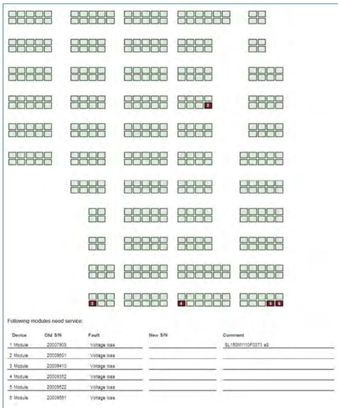
The SunSniffer® intervention calculator shows exactly which modules are defective and should be changed - and, how much this action would cost and how much yield would be wasted if not fixed. The settings can be adjusted individually. You see exactly, when the investment of new modules will pay off: the point, when additional profit starts to accumulate.
