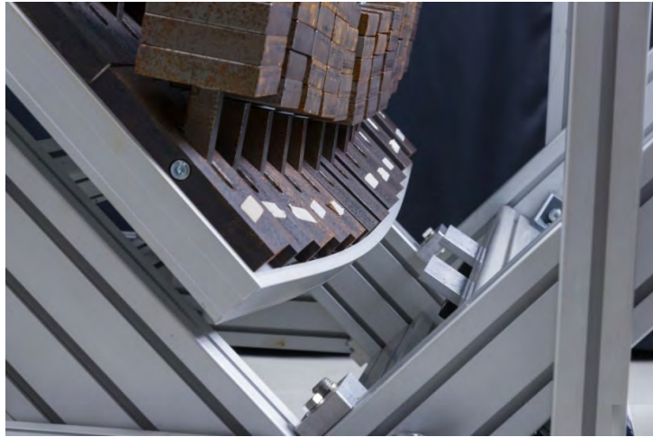
Figure 7.2.1: New test apparatus for snow load testing at TÜV Rheinland 2012: Application of load elements causing the bending of a PV module frame.
