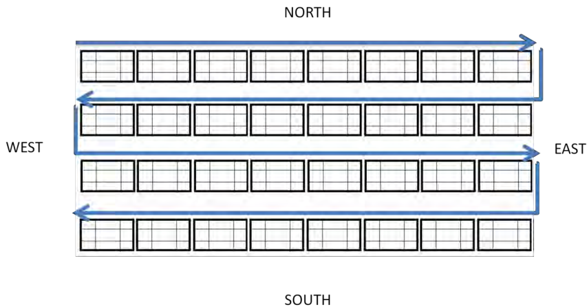
Figure 35: Recommended walking direction of a single-rowed module construction.
