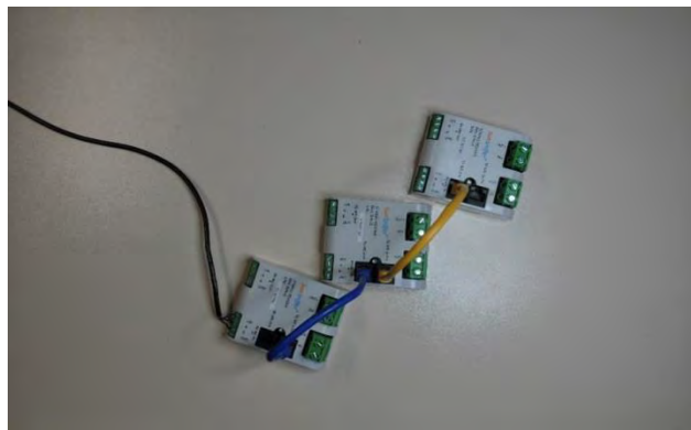
Figure 9: String Readers connected in series via RJ-45.
